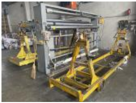
Reference: STV-001 PREPARATION MACHINE FOR A-FRAME Year: . Brand: . Width: 3400mm
